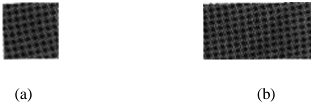
Fig 3-6 Turning a square (a) into a rectangle (b) with scaling factors s_x = 2 and s_y = 1 .
